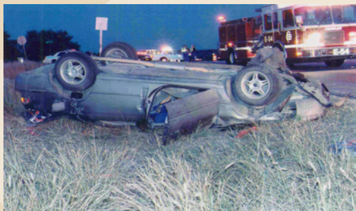
The roof on the driver's side crushed nearly 18 inches and impacted the driver's headrest. Ms. Green was pinned in the driver's seat.
